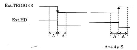
Fig. 8. External trigger and HD relations
